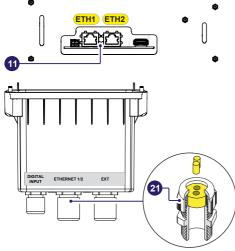
⚠ ATTENTION – If the inverters need to be connected in daisy chain or ring configuration use both connectors.
