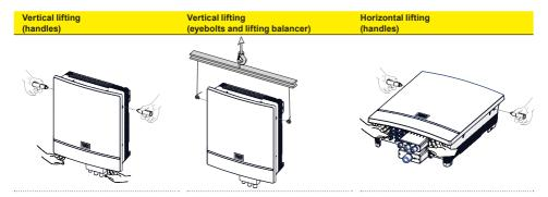
⚠ ATTENTION – DO NOT grab the equipment from the rear flange! Risk of injury due to cutting surfaces and risk of equipment damage. Always use proper lifting equipment!
