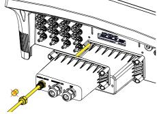
•Install the 2 poles screw terminal block (supplied) on the cable (see paragraph "3.5.2 Tightening torques").
