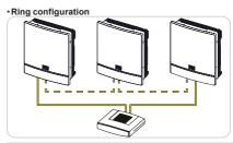
POTE - In case inverters are connected to the networking switch with a ring topology is recommended to enable SPT protocol on the switch (Spanning Tree Protocol SPT (IEEE 802.1D) is enabled by default on inverters.
