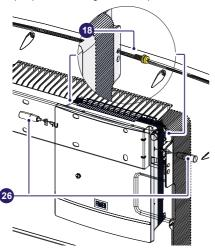
•A padlock can be installed to lock the inverter to the bracket so that it cannot be disassembled by outsiders.
