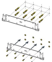
· Attach the bracket (05) to the support.
